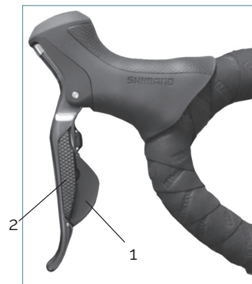
Fig: Left lever 1) "Down" gear 2) "Up" gear
