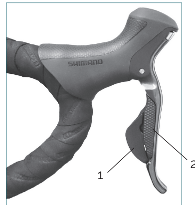
Fig: Right lever 1) "Down" gear 2) "Up" gear
