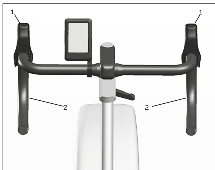
Fig: Shifters right side 1) shifters 2) Sprint button
