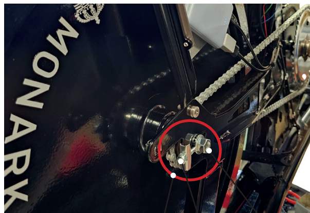
Fig: Chain adjustments 2 1) Chain adjuster 2) Chain adjuster nuts 3) Axle nuts
