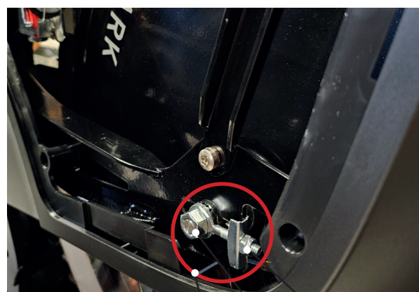
From the left side 1) Chain adjuster 2) Chain adjuster nuts 3) Axle nuts
