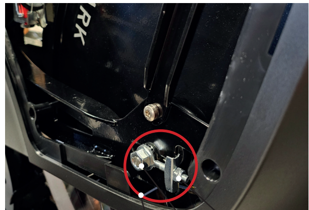
From the left side 1) Chain adjuster 2) Chain adjuster nuts 3) Axle nuts
