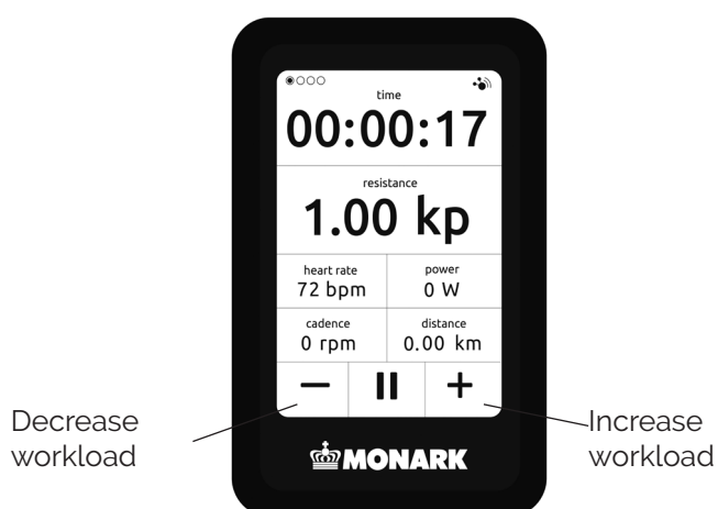
Fig: Workload in kilopond
