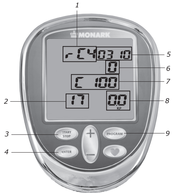
Fig: Display 'Calibration mode' 1) Bike model 2) Current potentiometer value 3) START STOP 4) ENTER 5) Software version 6) Hours in use 7) Cycle constant (1.00) 8) Calibration point 9) PROGRAM
