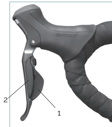
Fig: Left lever 1) "Down" gear 2) "Up" gear
