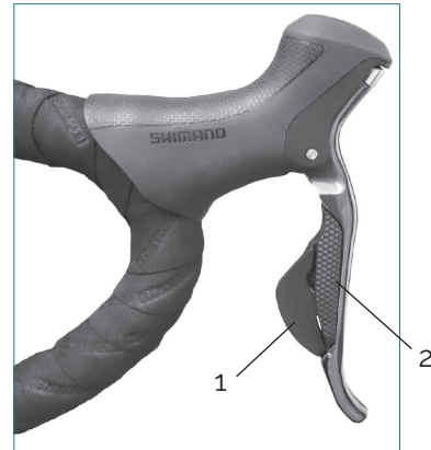
Fig: Right lever 1) "Down" gear 2) "Up" gear
