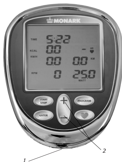
Fig: Workload adjustment and connections 1) USB 2) Workload adjustment (+/-)
